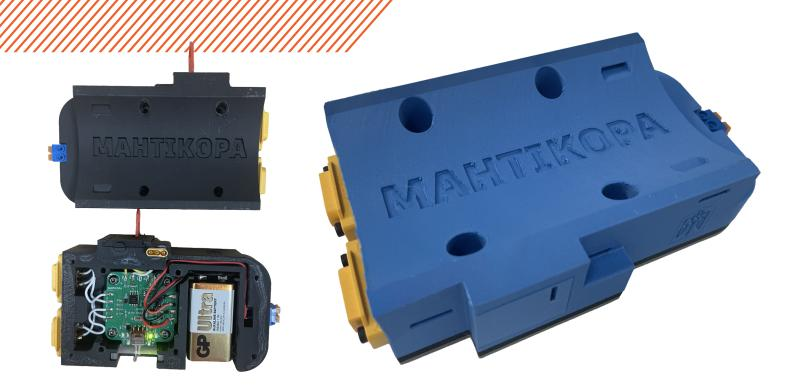
The drones are supplied together with the **Manticore Munition Initiation Board (MIB)**, which is designed and manufactured by the Research and Development Department for the development of UAV onboard equipment of **PJSC STC "Electronprylad"** and serves to initiate the detonator's explosive reaction into the munition.
